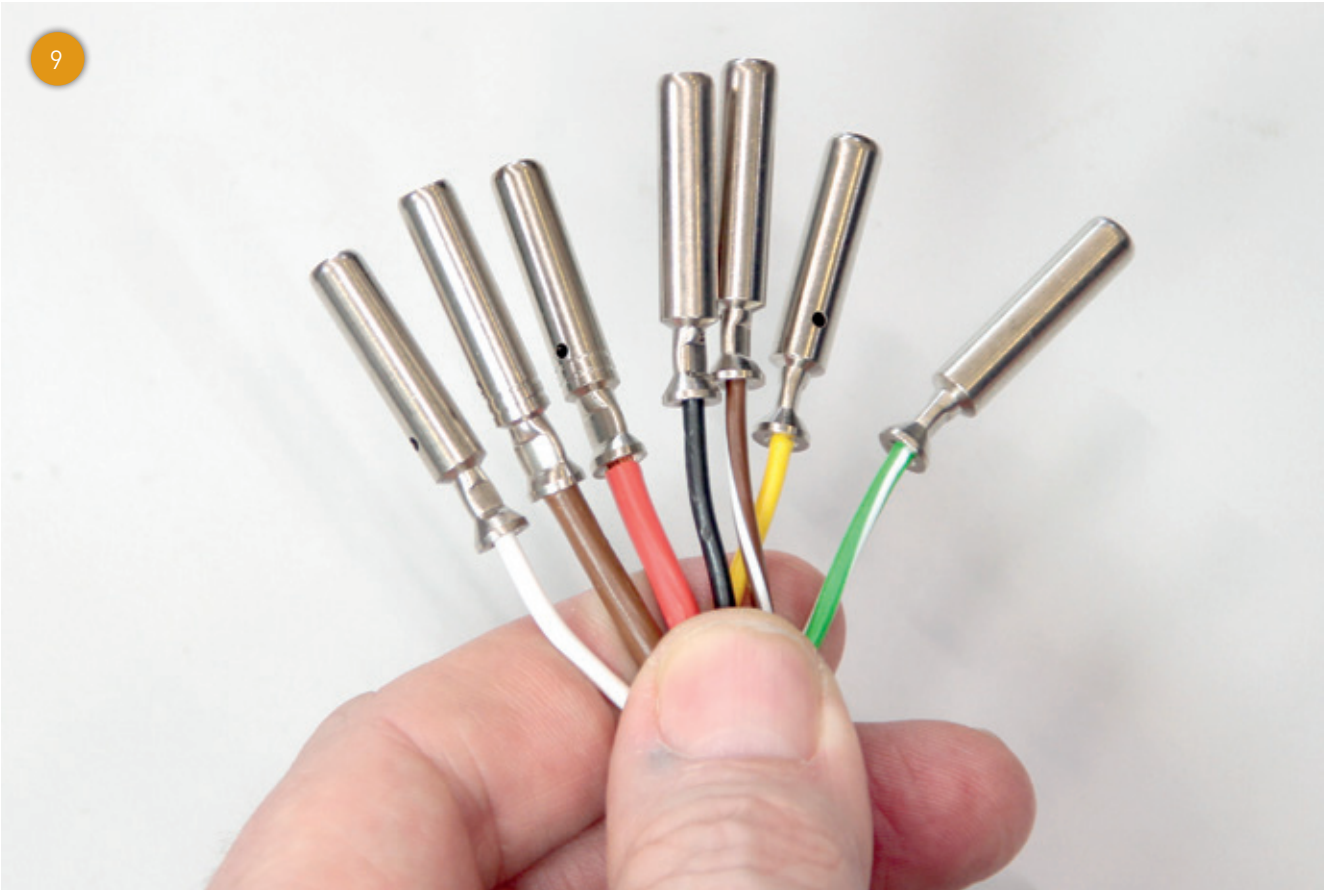
The finished crimp contacts look like this.
