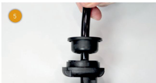
5 First, strip the vehicle cables to a maximum of 5 mm with a suitable tool. To prepare the plug connection, first push the end cap...
