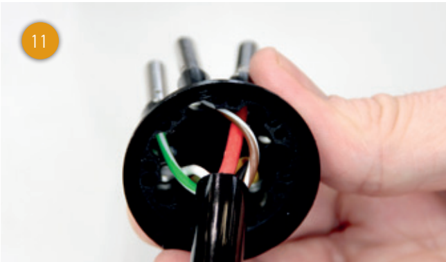
Insert the crimp contacts in the insert connector in accordance with the connector layout diagram.
