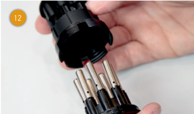
The first plug housing is placed on the insert connector. It must click into place audibly.
