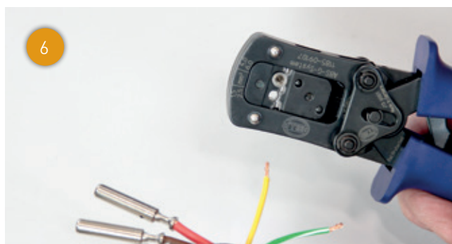
6 ... and then the cup seal onto the cable. Place a crimp contact of the appropriate size for the cable diameter in the pliers.
