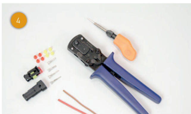
4 These are the materials required to produce a SUPERSEAL plug connection.
