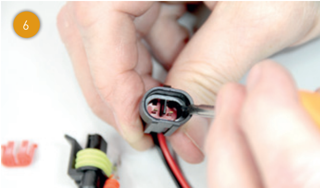
....prise out the secondary fuse.
