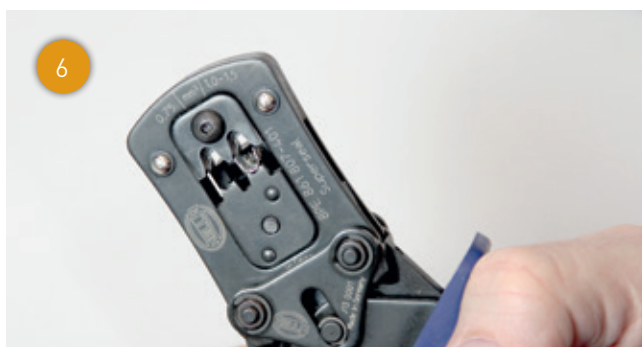
6 Then place the socket contact in the positioning aid of the pliers. Ensure that the socket contact is flush with the front of the tool.
