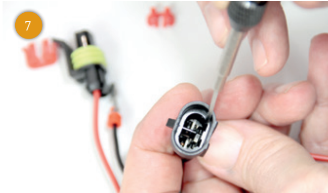
Here you also have to unlock the locking tab on the contact pins...
