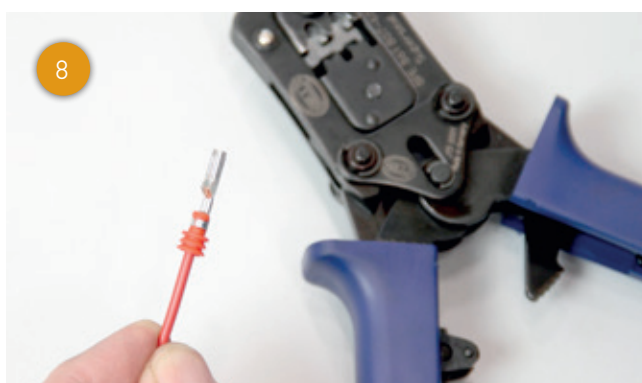
8 It is important that the cable, socket contact and seal are positioned correctly in the tool.
