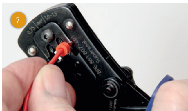
7 Now insert the cable with the seal and crimp the socket contact.
