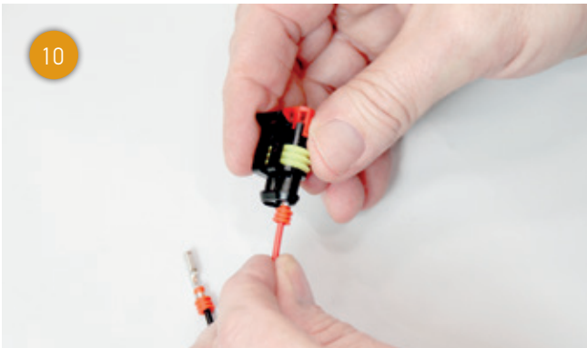
Now insert the crimped socket contact into the socket housing...
