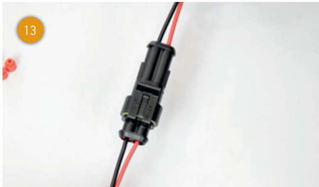
Putting the plug connection together in this way ensures that it is dust and waterproof.
