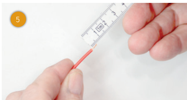
5 First, strip the vehicle cable to a maximum of 5 mm with a suitable tool. Slide on a seal to fit the cross-section of the cable.
