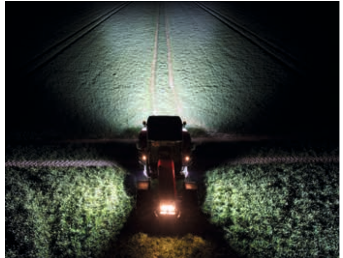
The significantly improved light output after converting to LED headlamps. The current consumption has been significantly reduced and is now 41.4 amperes.
