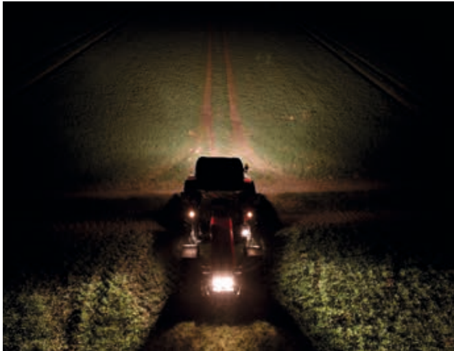
The light output with conventional halogen headlamps before the conversion. The current consumption here was 60.9 amperes.
