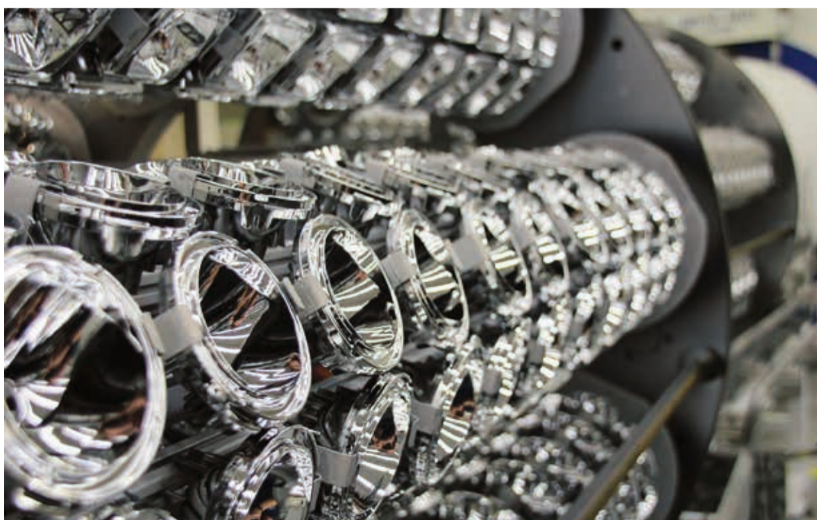
The reflectors are given their shiny surface coating in the vacuum chamber.
