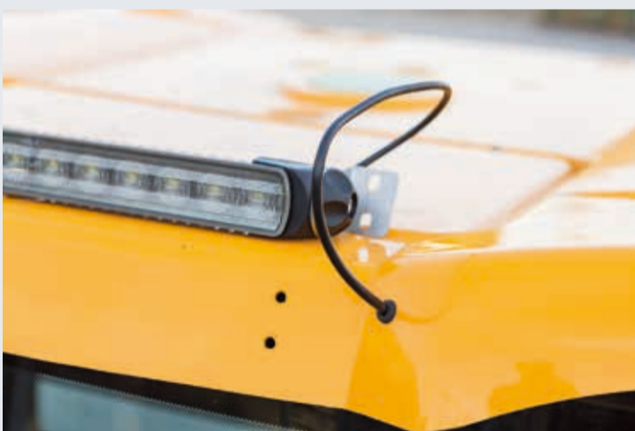
An LED light bar/work light has been mounted with a universal bracket set: here the universal bracket can be seen already secured on the side.
