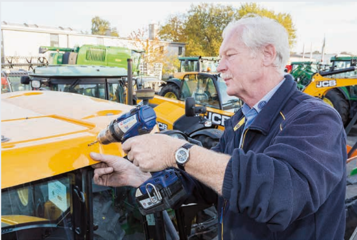
Mounting A Light Bar On The Roof: Dietmar Bengsch in action with the drill after using a template to measure requirements.
